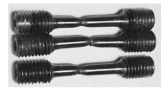
Figure 1. Ruptured samples after the tensile limit test (St12T steel, temp. 400 °C).
