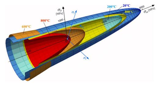
Figure 5. St12T plastic region paraboloid distribution, created using the Burzyński approach [30].
