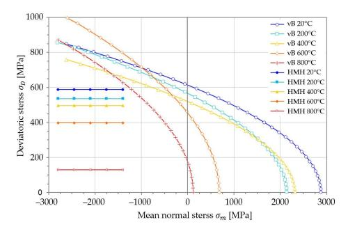
**Figure 6.** Comparison between HMH hypothesis and validated Burzyński hypothesis (vB) for St12T steel including a set of elevated temperatures [30].
