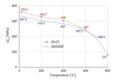
**Figure 3.** Tension elastic limits for two key heat-resistant steels (St12T and 26H2MF) at elevated temperatures (26H2MF curve added only for reference).
