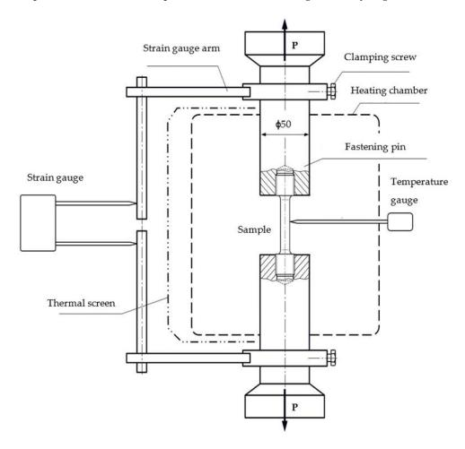
Figure 2. Experimental setup used for tensile and compressive limit tests.
