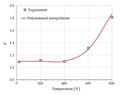
Figure 4. St12T steel elastic region asymmetry coefficient vs. temperature [30].
